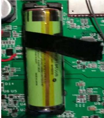
To make it easier to remove the battery, a Puller can be made up using a piece of ribbon: cut an 80mm length of 8 to 12mm wide ribbon. Fold in half and glue the last 20mm of each end together with superglue. Once the glue is dry, you can sleeve the ribbon over the battery. The end of the ribbon can then be used to lift the battery out of the holder.
