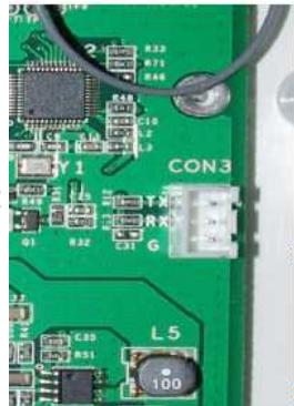
The JST plug is polarised so it will only go in one way. Plug the header from your adaptor cable in to this socket and open the Console.
