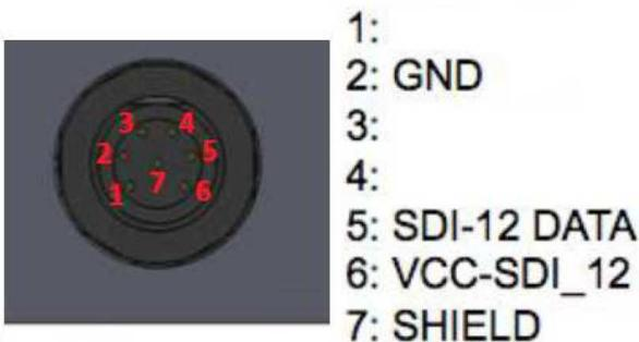
This image is taken looking at the socket on the TBS12 body face on. If you plug the 7 pin plug into the socket and stand the unit on its head so the connector is on top, the orientation will be the same when you look down on the back of the plug from above (after taking off the backshell)
