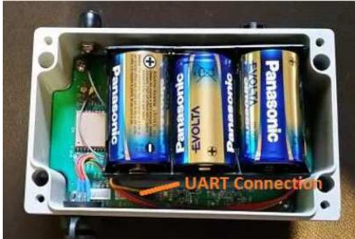
The JST plug is polarised so it will only go in one way. Plug the header from your adaptor cable in to this socket and open the Console.
